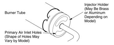
Figure 20 - Injector Holder On Outlet Burner Tube
